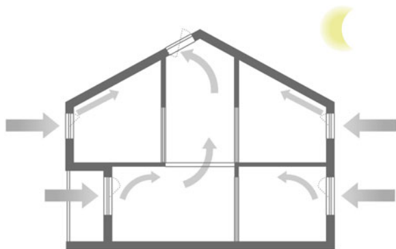
Fig. 2.23 Convective nighttime cooling by means of ventilation
