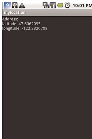
Figure 10.3 Geocoding example, which converts an address string into a latitude-longitude coordinate.
