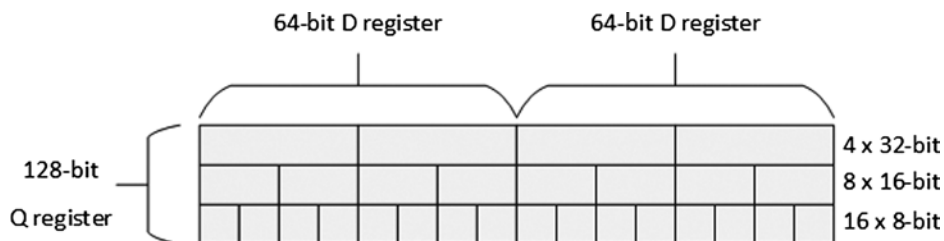
Figure 14-1. NEON registers and data types
