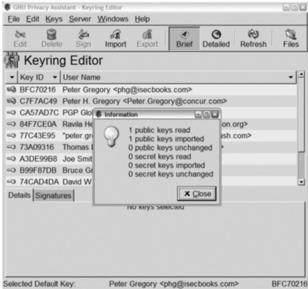
Figure 5-15 Importing a public key using GnuPG
