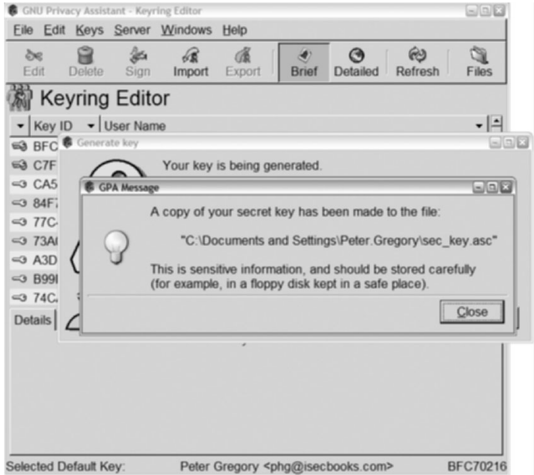
Figure 5-14 Creating a public-private keypair using GnuPG
