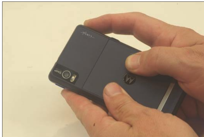
Figure 1-1: Thumb-placement suggestion for removing back cover.
