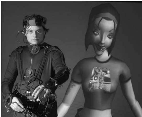
Figure 9.14 Sensors adorn the actor's body (Courtesy: Kevin Monko, Thinkframe). (See Plate XVI.)
