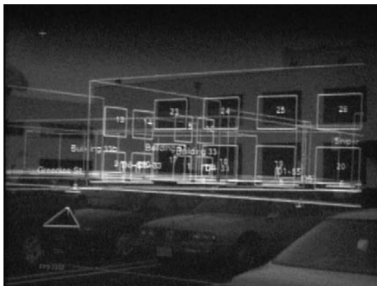
Figure 9.12 Outdoor AR-battlefield augmented reality system (inertial GPS technology) (Courtesy: The Advanced Information Technology Branch of Information Technology Division at the Naval Research Laboratory, US Navy). (See Plate XIV.)
